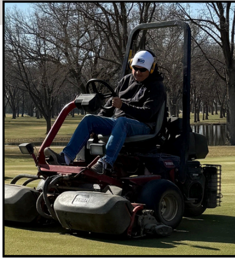
Eric and his team have mowed the greens three times already in preparation for the 2025 season. This particular mower is the 2013 Toro Reelmaster with 3,100 hours on it.
